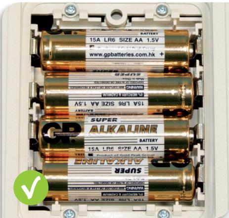
If batteries are inserted make sure they are the correct way round
